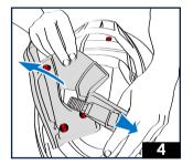
4 - Completely remove each of the cheek pads from the inside by sliding them onto each end of the chinstrap while turning the helmet over if necessary.
