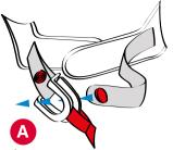
WARNING! Never use the ring as the only way of fastening the chinstrap. In order to be properly tightened, the chinstrap must pass through the double-D ring straps as instructed. Improper use of the chinstrap can cause your helmet to be thrown off in an accident, leaving your head unprotected. Try to pull on the chinstrap with your fingers. If the strap loosens in any way, you have not fastened the chinstrap properly in the
