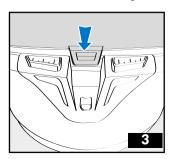
3 - Lower the visor until the central visor grip comes to stop (without forcing) against its lock button.
