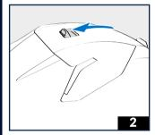
1 & 2 - To use the upper vent, move the button backwards (open) (1); forwards (closed) (2).
