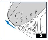
2 – Hold the visor in its raised position in front of the side plates and bring it to rest against the visor step on either side.
