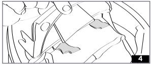
$4\,$  – The Morpho Pad has now been removed. The comfort liner can be re-installed, see p. 20.
