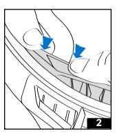
2 - Make sure that the anti-fog mask is correctly clipped into place.
