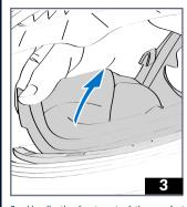
3 - Un-clip the front part of the comfort liner, clip by clip, by pulling inwards starting from either of the two ends.
