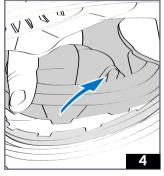
4 - The comfort liner is completely detached and can now be removed.
