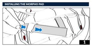
1 - Slide the Morpho Pad through its two securing straps.
